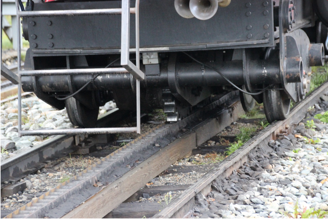
A view of the locomotive's cog wheel engaged in the cog track.
