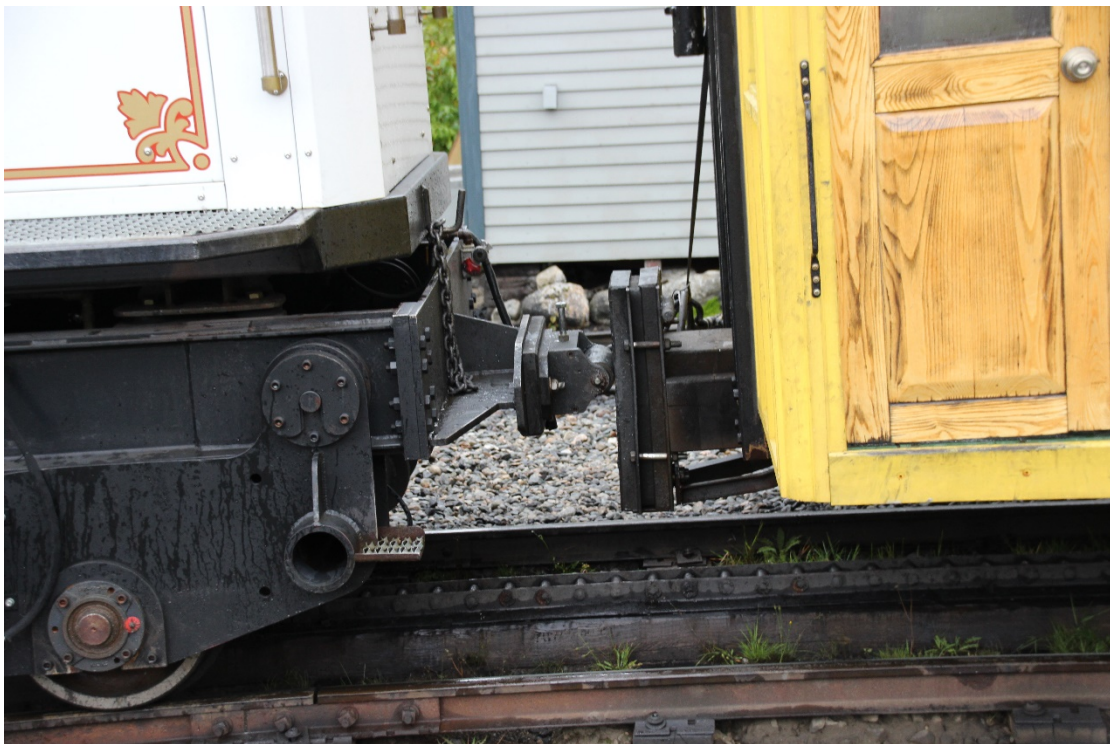
Note the small bumpers between the locomotive and coach; no coupler to hold the two together, just gravity at work.
